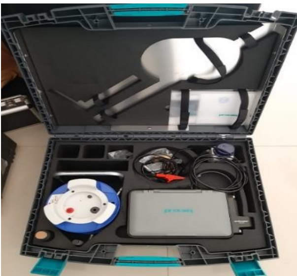
Gambar 1. Set half cell potential tester
