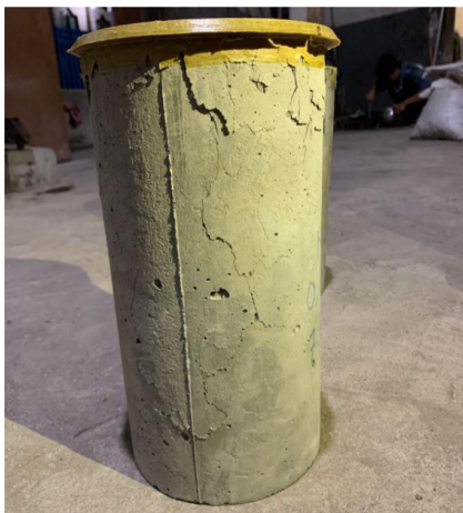
Figure 1. Crack patterns observed in one of the concretes we used for testing.
